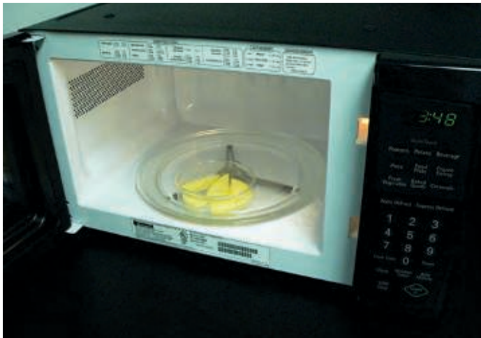
Measuring mango dry matter content with a microwave oven
