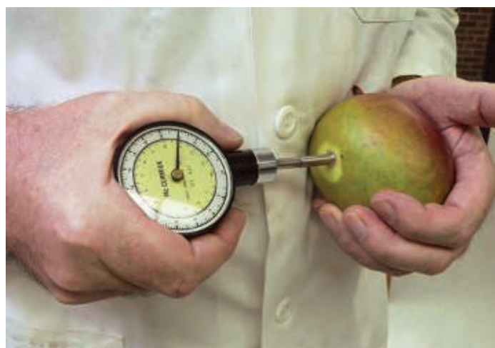
Measuring mango flesh firmness with a penetrometer
