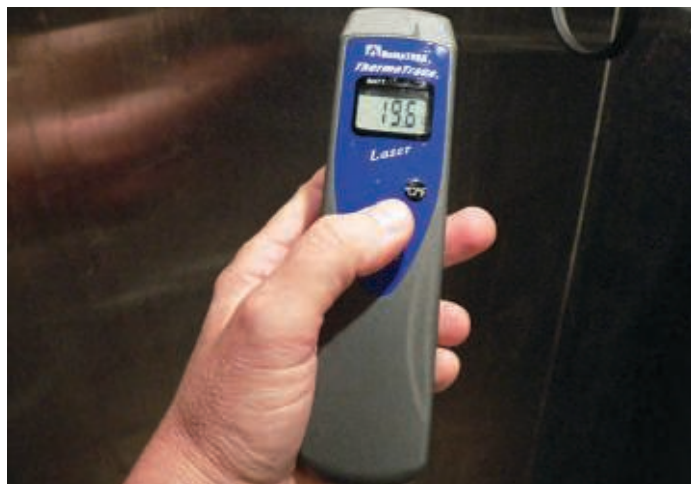
Measuring surface temperature with an infrared thermometer
