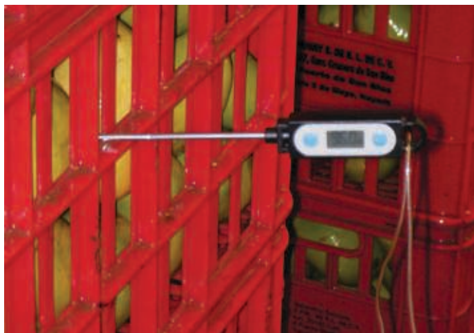
Measuring mango flesh temperature following hydrocooling
