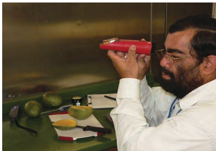
Measuring mango fruit TSS with a refractometer
