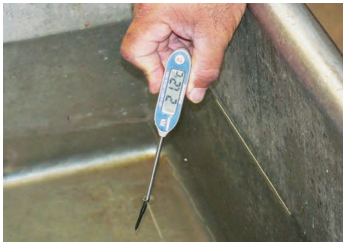
Measuring hydrocooler water temperature
