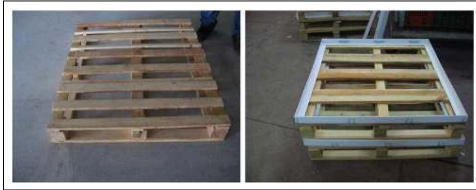
Figure 5: Wooden Stringer Pallet
