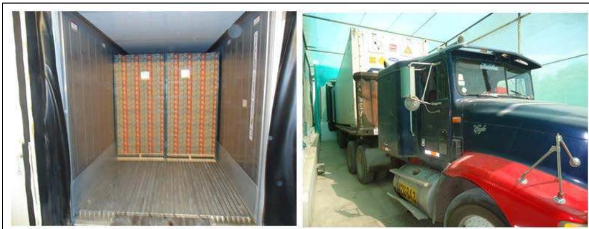
Figure 7: Palletized Loads Inside Pre-Cooled ISO Intermodal Container
