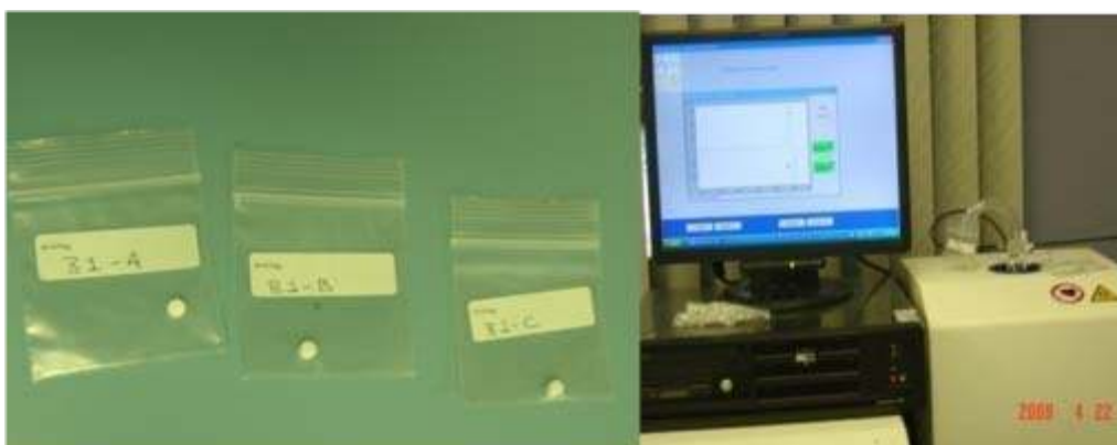
Alanine dosimeters and Electron Spin Resonance equipment used to measure the absorbed dose
